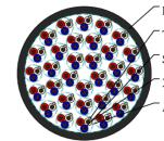
LSOH (SHF1) Outer Sheath Tinned Copper Drain Wire Stranded Copper Conductor XLPE Insulation Al/polyester Tape Screen
